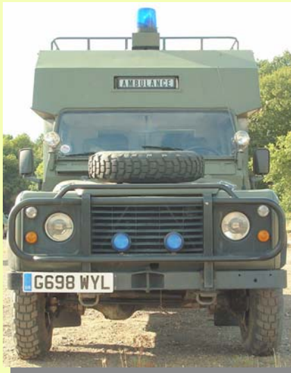
Front of the same vehicle showing the slab-front of the Locomotors design, compared to...
