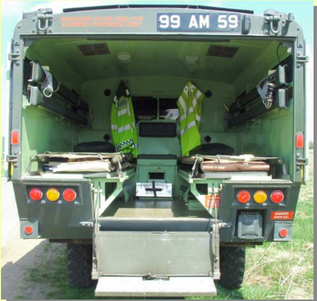
First Generation internal layout. Earlier SII-based versions has a water container locker above the bulkhead window. RAF versions have the mains input socket (lower right). Unit under attendant's seat contains a sink and the heater matrix. (Mike Allmeij)
