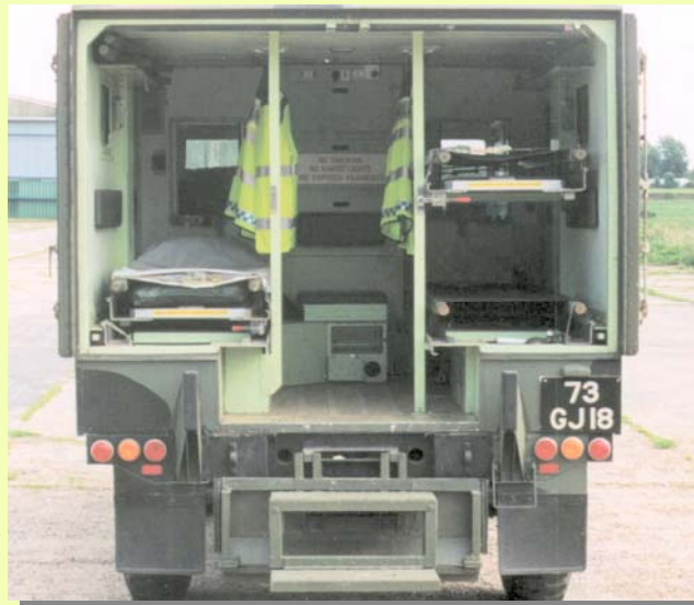
Rear saloon of the 101 Ambulance. Two-over-two stretcher configuration with mechanised lifts, central storage locker, on-board thermostatically-controlled heating and even a chance to watch where you're being driven to. (Mike Allmeij)
