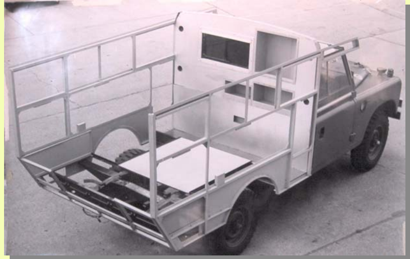
In the raw: Dutch-spec SIII 109" showing the basic construction details of a Marshall body. Marshalls / Wayne Davies
